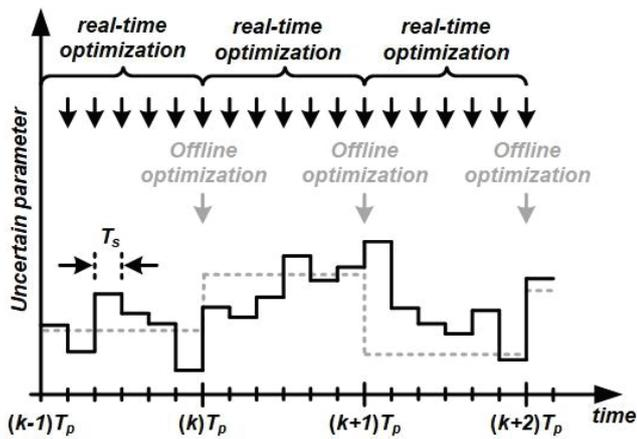
Figure 1: Offline optimal power flow (gray) and online optimal power flow (black).
