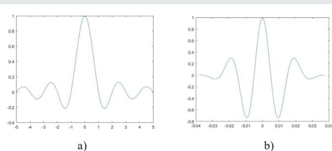
Figure 1: Rice. 1. Signals characterizing the (a) absence of and (b) the presence of a defect.
