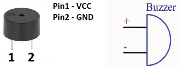
Figure 7: Buzzer & Its Pinout. Image source: Non-copyrighted Google Image.
