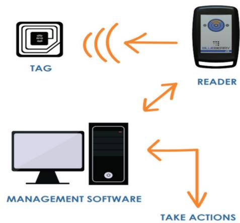
Figure 10: Process of RFID. Image source: Non-copyrighted Google Image.
